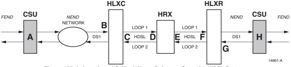
Figure 103-1. Location of Critical Alarm Points on Soneplex HDSL System
